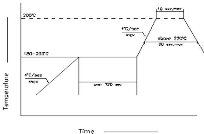
1. Reflow soldering should not be done more than two times. 回流焊不可以做两次以上
